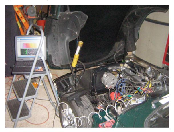
With the basic system operation verified and the connections understood, what remained to accomplish was to mount the EDIS module, MegaJolt box and coil pack and make a wiring harness to connect all the components permanently. I decided to mount the EDIS module and MegaJolt box in the driver's foot well area, as indicated in the following photos:
