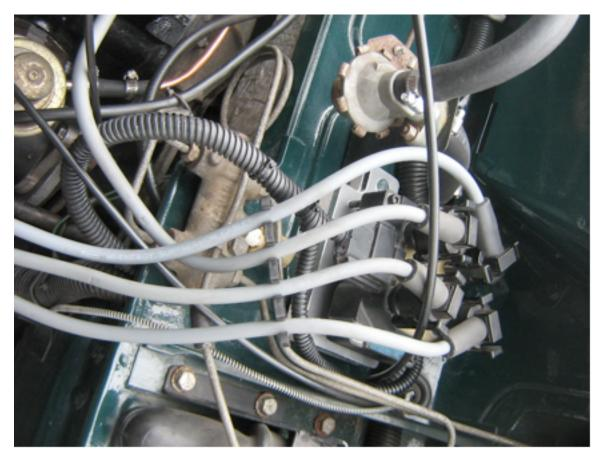
A set of 1991-96 Ford Escort spark plug wires work perfectly well to connect the coil pack to the spark plugs.
