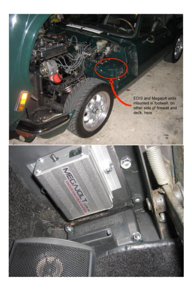
The MegaJolt box needs to be mounted in a protected environment, and locating it and the EDIS module close together reduces wire lengths and minimizes the chances for interference on the signals between them.
