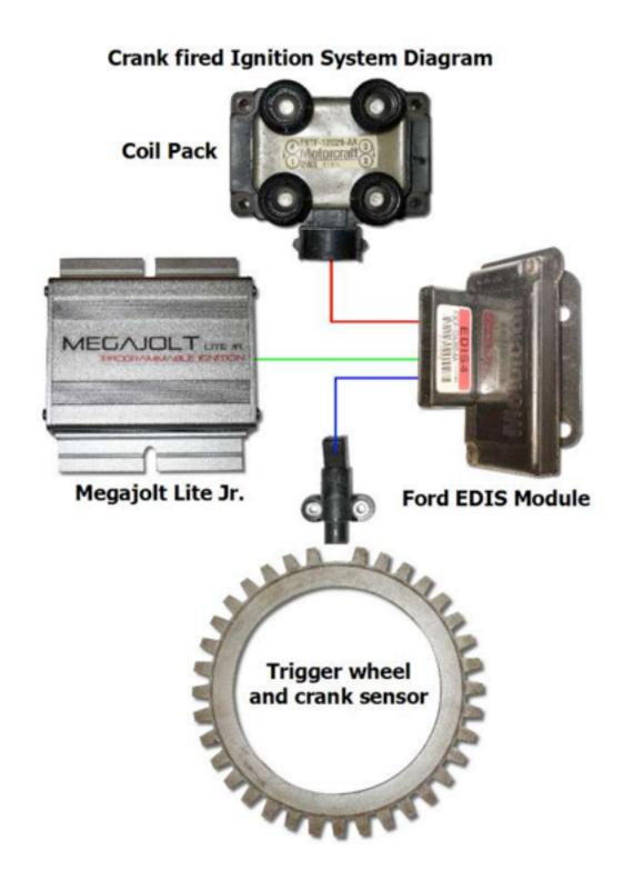
Here are the necessary components to convert a Spitfire or GT6 to MegaJolt:
